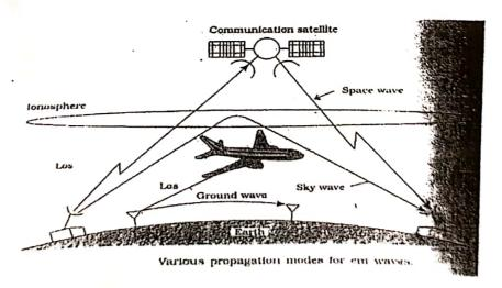
(c) Space wave propagation:-The space wave can travel through atmosphere from transmitter antenna to receiver antenna directly in the earth's troposphere region. The space wave propagation is utilized in very high frequency (V.H.F.) bands (between 30 MHz to 300 MHz). Ultra high frequency (U.H.F) bands and microwaves.
