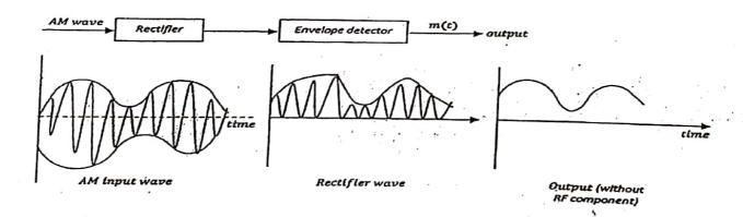
The modulated signal is passed through the rectifier to produce the output. The envelope of signal is the message signal. In order to retrieve m(t), the signal is passed through an envelope detector.
