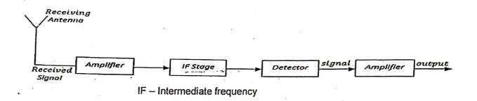
Detection is the process of recovering the modulating signal from the modulated carrier wave.
